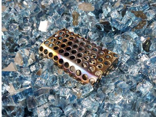
To ensure proper air flow, the protective screen requires to be clear of media on the surface and all four sides as shown above.
